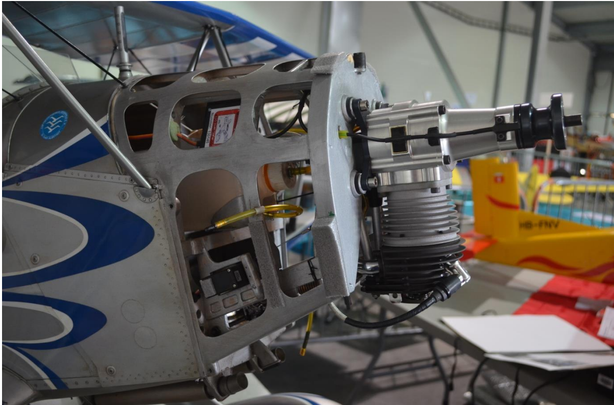
A peek under the hood of the winning Bucker Jungman. Engine is Fiala 70cc petrol four stroke. Note the sponge pads arranged to keep the cowl from direct contact with the front engine mount bulkhead.
